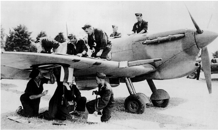
One of No. 1 Fighter Wing's Spitfire VCs undergoes maintenance shortly after its reassembly at RAAF Base Laverton, Victoria, in early 1943. Like many other Spitfires sent out from Britain at this time, the aircraft is still wearing its factory-applied two-tone Desert camouflage scheme. They were soon painted in more appropriate colours and had unit codes added prior to their flight north to Darwin. (Andrew Thomas Collection)
