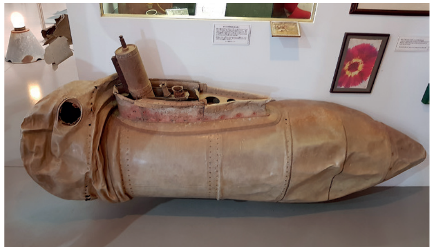
A 94-gallon drop tank from a Zero-sen, which was jettisoned over northern Australia prior to the fighter entering combat with No. 1 Fighter Wing Spitfires. This tank was more than twice as large as the 30-gallon drop tank used by the considerably shorter-ranged Spitfire VC. [Author's collection]
