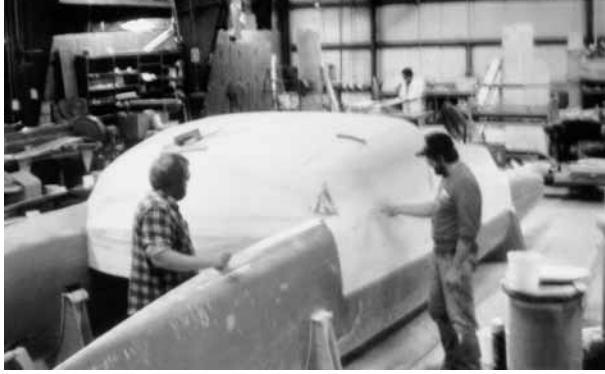
Figure 3-2 A plug can be built of any combination of easy to shape materials. This catamaran plug's cabin area was shaped in Styrofoam™ and then faired with epoxy/407.
