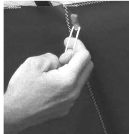
Figure 8 Insert Under Surface Battens
