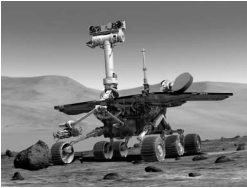
Figure 1.9: Robotic systems. (a) Spirit, one of the two Mars Exploratory Rovers that landed on Mars in January 2004. (b) The Sony AIBO Entertainment Robot, one of the first entertainment robots to be mass-marketed. Both robots make use of feedback between sensors, actuators and computation to function in unknown environments. (Photographs courtesy of Jet Propulsion Laboratory and Sony Electronics, Inc.)
